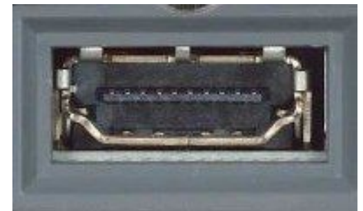
Złącze HDMI (High Definition Multimedia Interface)
